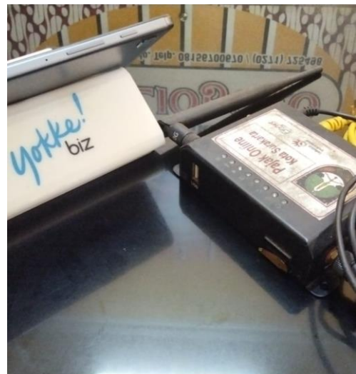
Gambar 3.15 – Kegiatan Pemasangan alat TMD ( Terminal Monitoring Device )
